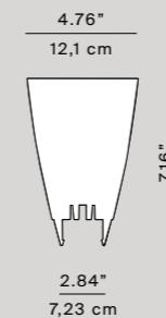
Polycarbonate diffuser for halogen
