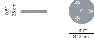
D13G.air/4 fixed base for dowels
