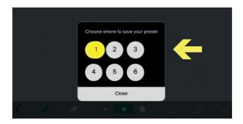
On this screen you can save your composition by pressing one of the six boxes. If the box is yellow, a preset has already been saved in that position. Otherwise, the box will be white. To exit, press the "close" button.
