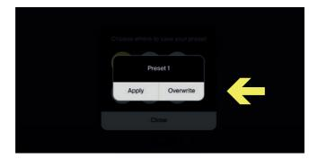
If you press a box with a saved preset, a drop-down menu will appear that will allow you to apply the previously saved preset -"Apply" - or overwrite the preset with the one you have just created - "Overwrite".
