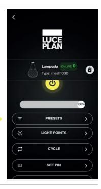
Pressing the "Presets" button will display a screen for activating presets.
