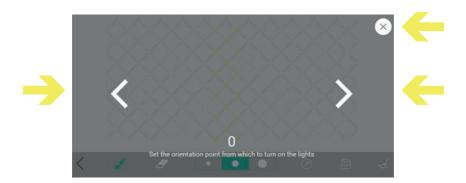
Using the arrows, you can set the centre line of the lamp. Each time the arrows are touched, the lamp will light one column of light points corresponding to the relative centre of the lamp. To save the setting and exit the screen press "X".
